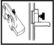
The Elevator Bolt Locking System is used on top trays on Best easels. The 2 metal plates and round plastic guide keep the parts parallel which
