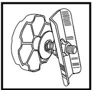
Height & tray adjustments unlock easily, yet lock into place & stay locked because of the Wedge-lok System. The metal plate features wedge-cut edges that conform
